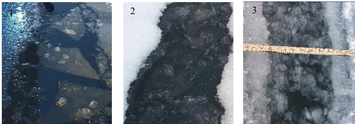
Figure 7. The sequence of brash ice formation during test 1. The figures illustrate the top view and underwater view. Photos 1 to 3 show the top view: after 2 nd ; before 10 th and after 12 th BE, and 4 to 6 shows the underwater view: after 1 st ; 3 rd and 13 th BE.
