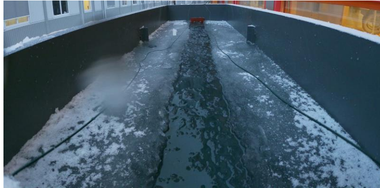
Figure 2. Example of the brash ice channel formed from exposure to the outside meteorological condition.
