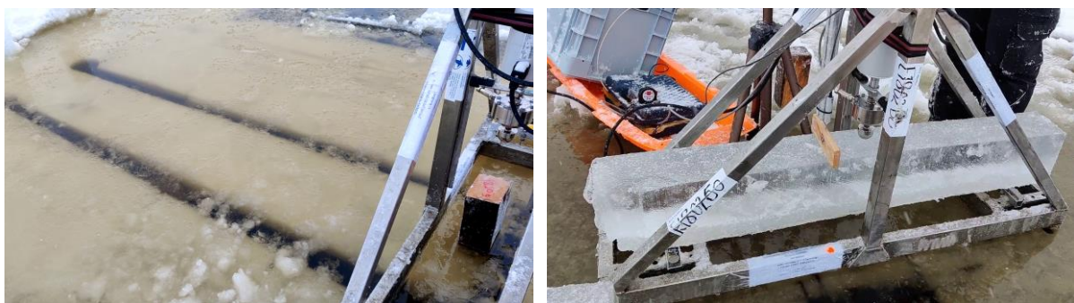
Figure 1. Cantilever beam test (on the left) and ex-situ 3-point bending test (on the right).
