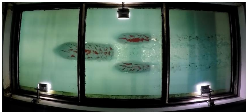
Figure 3 – Ice breaking by model hulls at 0.36 m/s (5.0 knots full-scale)
