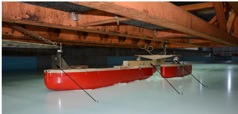
Figure 1 – Model test of multi-hull icebreaker in ice basin (1 –towing dynamometer; 2 – frame bridge to connect hulls; 3 – five-component dynamometer to measure ice load on wing hulls)
