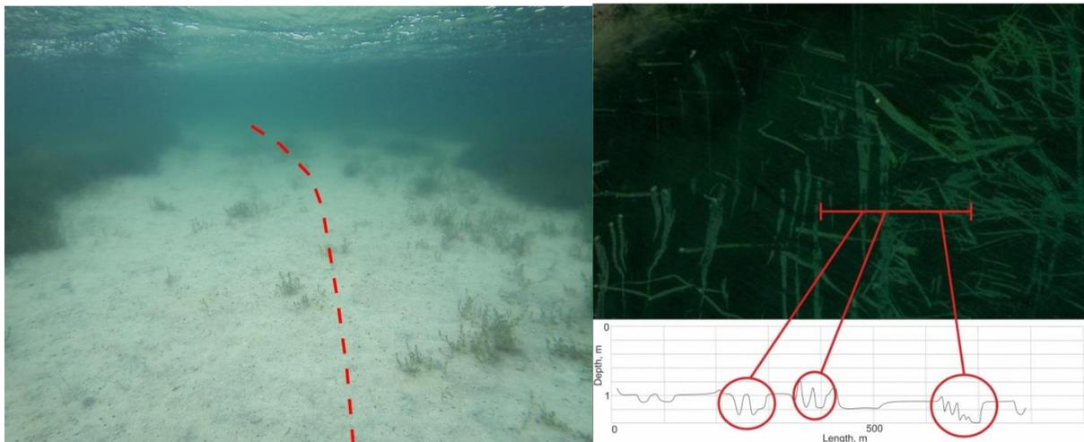
Figure 3. At the left: an underwater snapshot of ice scour (red line shows an axis) near Morsky Island; at the right: an echo sounding profile on a WorldView-3 image mosaic (spring 2020)
