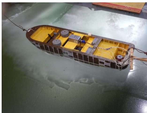
Figure 2. Model tests of the IRSPP in the ice tank
