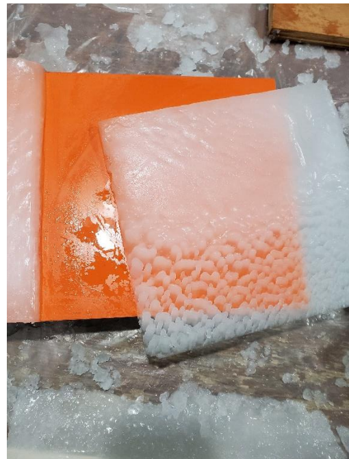
Figure 10. A photo of board 3 illustrating how a substantial portion of the spray-ice layer, that was melt-separated from the rest of the layer, had been easily slid off the board by hand when a relatively small shear force was applied at its edge. The portion was then placed back on the board in order to take the photo. Remnants of the thin brine layer that prevented solid-solid bonding of the ice to the board, and facilitated the slippage, can be seen on the board where the ice had previously been.
