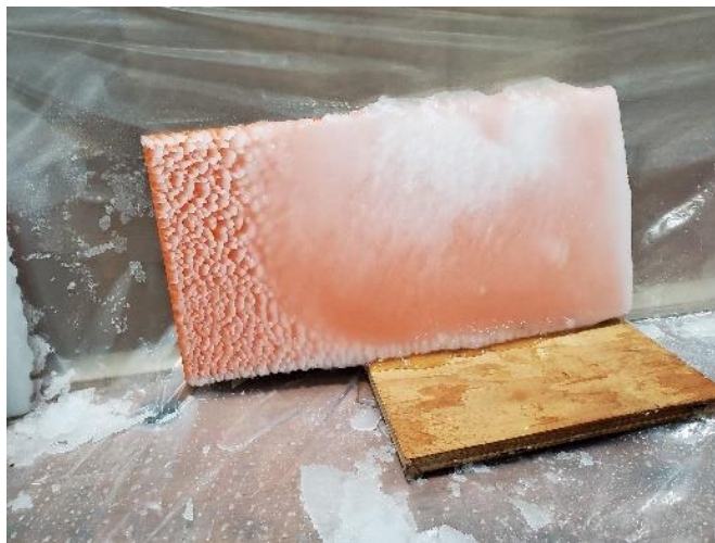
Figure 9. Board 3 with an accumulation of saline spray-ice. The icing layer was applied when the board was lying horizontally. Shortly after that the board was oriented vertically with its side-edge resting on a sheet of plywood. Within a few minutes substantial brine had drained from the icing layer and accumulated in a pool on the plywood at the base of the board. White regions of the icing accumulation indicate areas where some brine had drained out of the ‘spongy’ ice matrix.
