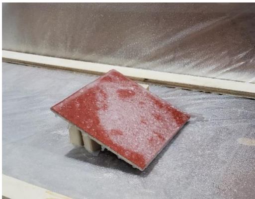
Figure 5. A freshwater ice layer resulting from spraying water onto a board with a red ice-phobic surface coating. The icing layer is of fairly uniform thickness (a few millimeters), however a significant portion of the layer has a whitish color, due to internal reflection, because that portion has delaminated/lifted from the coating. The rest of the ice layer maintained direct physical and optical contact with the coating so that its red color is visible through it. In this case the lifting mechanism was probably due to water freezing and expanding at the lower edge (and possibly far side-edge) of the board.
