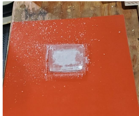
Figure 8. A fully prepared ice sample consisting of the snow-ice sample at the bottom and the ice plate at the top. A peripherally-wetted and frozen layer of snow provides a solid bond between the top and bottom ice components. The residual snow particles on the board from the preparation process will be swept off with a brush before the test.
