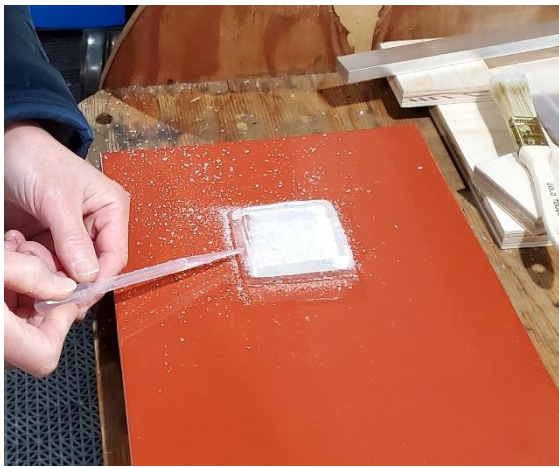
Figure 7. A dropper is used to wet the periphery of a layer of snow sandwiched between a snow-ice sample at the bottom and an ice plate on top.
