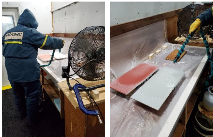
Figure 4. Spray-icing setup. (left) Boards 1 and 5 receive saline water spray from a manually operated spray nozzle in the Cold Room at an ambient temperature of -22\text{ }^{\circ}\text{C} . The nozzle is fed from a handheld pressurized container. The spray targets and nozzle are situated in the airstream of a fan (foreground) that generated a wind speed of \sim 1.1\text{ m/s} at the boards. The nozzle was activated and moved across the boards at roughly 10-20 s intervals. (right) Alternate view of the boards, with icing-layer accumulations, spray nozzle and fan (background).
