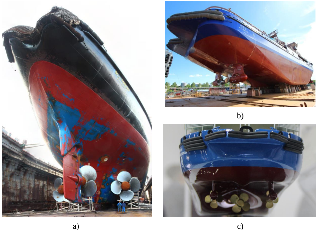
Figure 1 – Conventional icebreaker stern (a) and stern intended for podded propellers (b)
