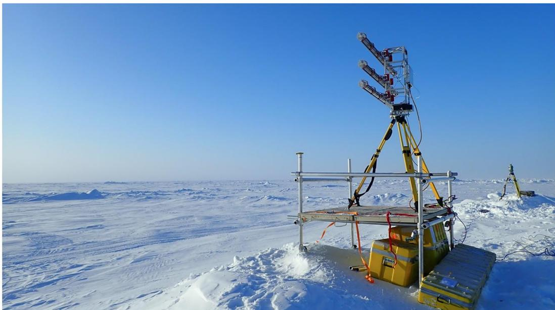
Figure 1. The Gamma Portable Radar Interferometer (GPRI) mounted on a multiyear ice ridge in the Beaufort Sea during a field campaign in 2020.
