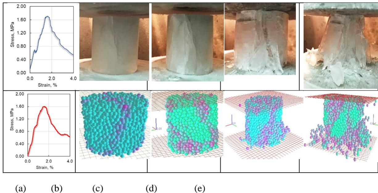
Figure 5. Experimental (top row) and theoretical (bottom row) deformation curves of compression of ice cylinders (a) and images of their destruction at different degrees of deformation (b - e)
