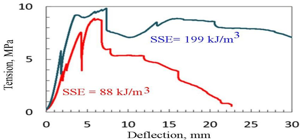
Figure 3. Deformation curves of the ICM beam reinforced with two basalt fiber layers: red line – without chemical modification, dark line – modified with the mixture of dispersed polytetrafluoroethylene, organosilicon oils and emulsions in a ratio 1:1:1, organosilicon oils and emulsions in a ratio 1:1:1
