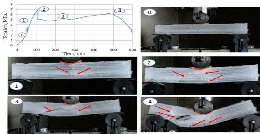
Figure 4. Deformation curve and cracking phases of the ice beam reinforced with two basalt layers in bottom and top zones
