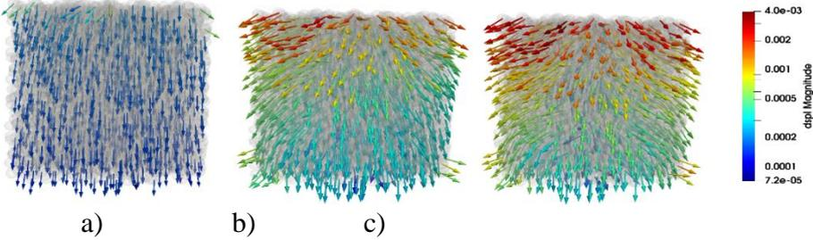
Figure 6. Moving elements in the model: (a)  $\varepsilon=0.52\%$ , (b)  $\varepsilon=1.57\%$ , (c)  $\varepsilon = 3.66\%$
