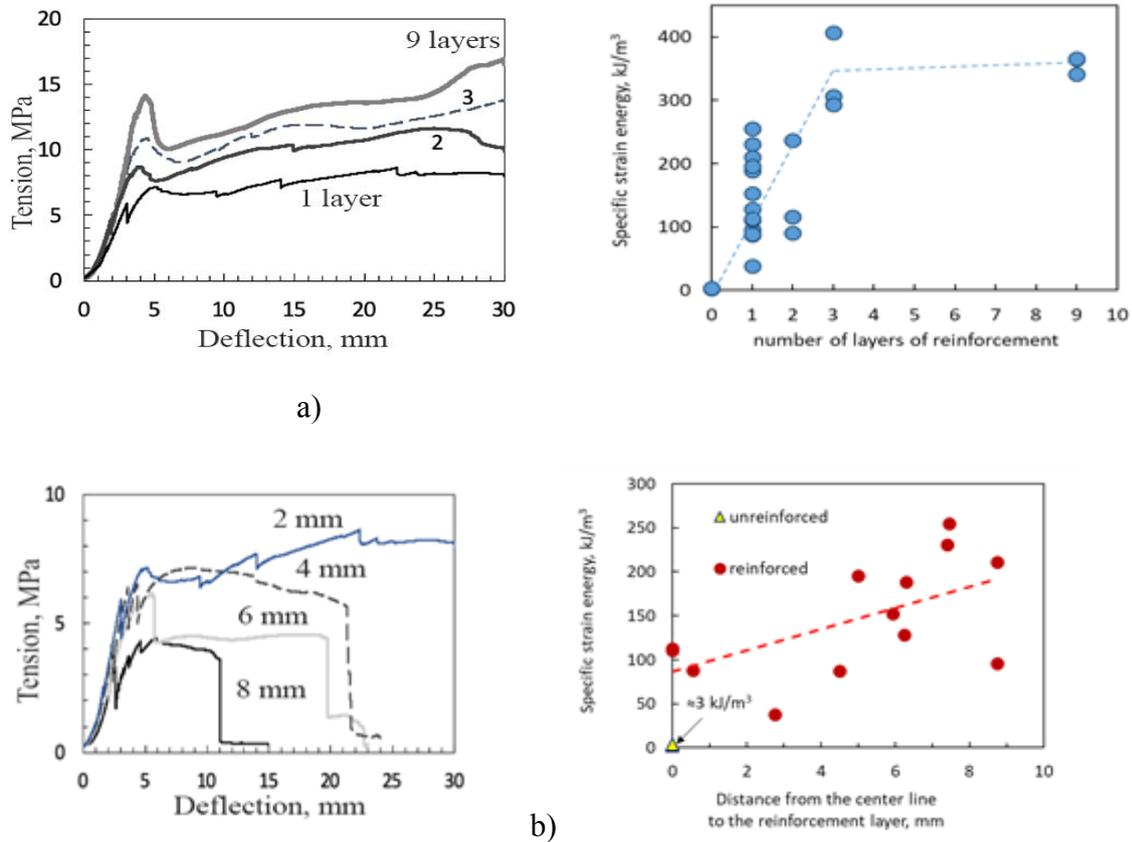
Figure 2. Nature of deformation curves of composite beams reinforced with basalt fibers, and dependence of specific strain energy (SSE) on the number of layers (a); deformation curves and SSE dependence on the location height of the reinforced layer in the ice matrix (b)
