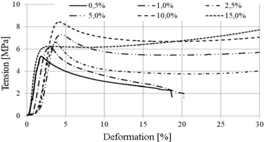
Figure 7. Ice cylinders with 10% sawdust filling subjected to axial compression at a speed of 3 mm / min (a) and 10 mm / min (b); a processed sample of an ice cylinder reinforced with hay (c) and deformation curves of composite ice cylinders for various concentrations (d)
