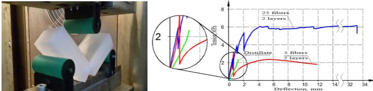
Figure 1. Image of a broken ice beam (a) and deformation curves of distillate ice beams b, green) reinforced with aramid fibers (b, read, blue)
