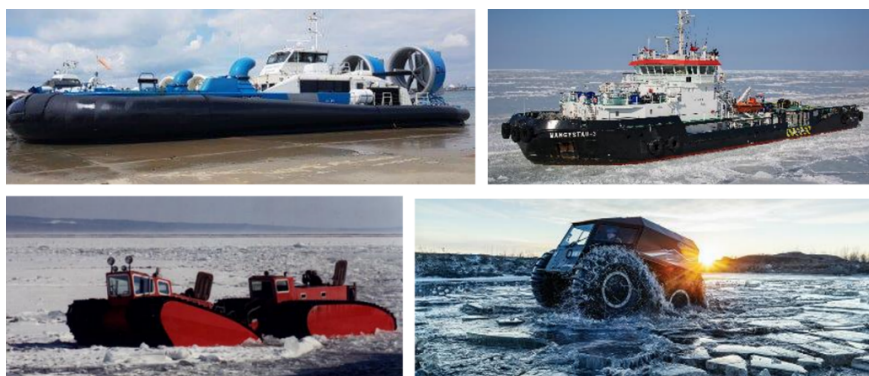
Figure 3 Top left: ACV Caspian Falcon (Length - 29.3-33.7m; Beam - 15m; Passengers - 130-180; Payload - 18-21 Tons.), Top right: IBSV Mangystau-2. Bottom left: ARKTOS utility
