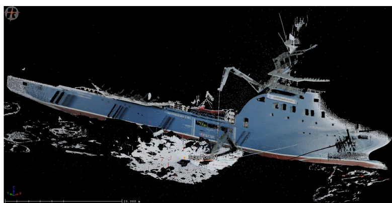
Figure 2. 3D point cloud, layered with photographs, obtained from laser scanning of ice floe 2.
