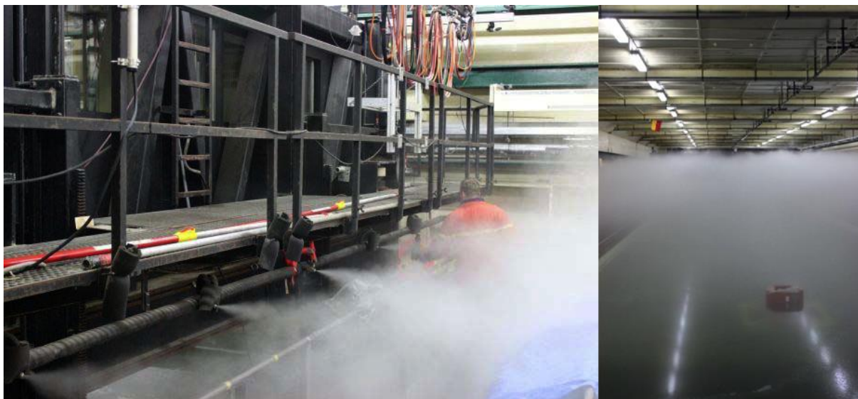
Figure 11. Water is sprayed by means of nozzles under high pressure into the air of the pre-cooled ice tank (left photo) where crystal nuclei are formed which settle down on the water surface (right photo).
