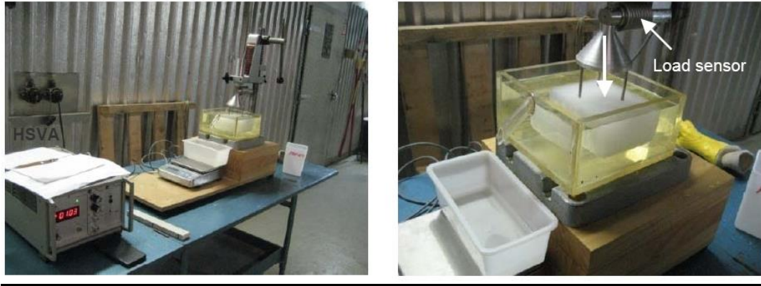
Figure 17. Set-up for determination of ice density
