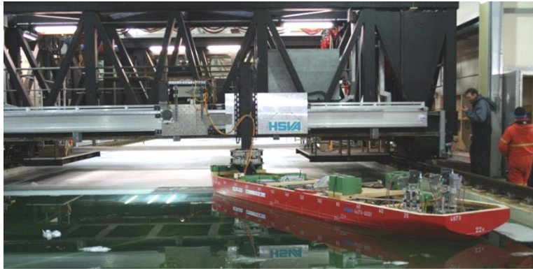
Figure 4. Transverse carriage installed as a sub-carriage on rear side of towing carriage.
