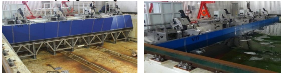
Figure 6. Removable flap type wave generator in Large Ice Model Basin.
