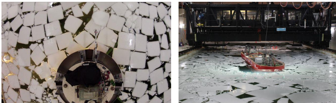
Figure 23. Model of a moored conical drilling platform (left) and ship model (right) in broken ice conditions.
