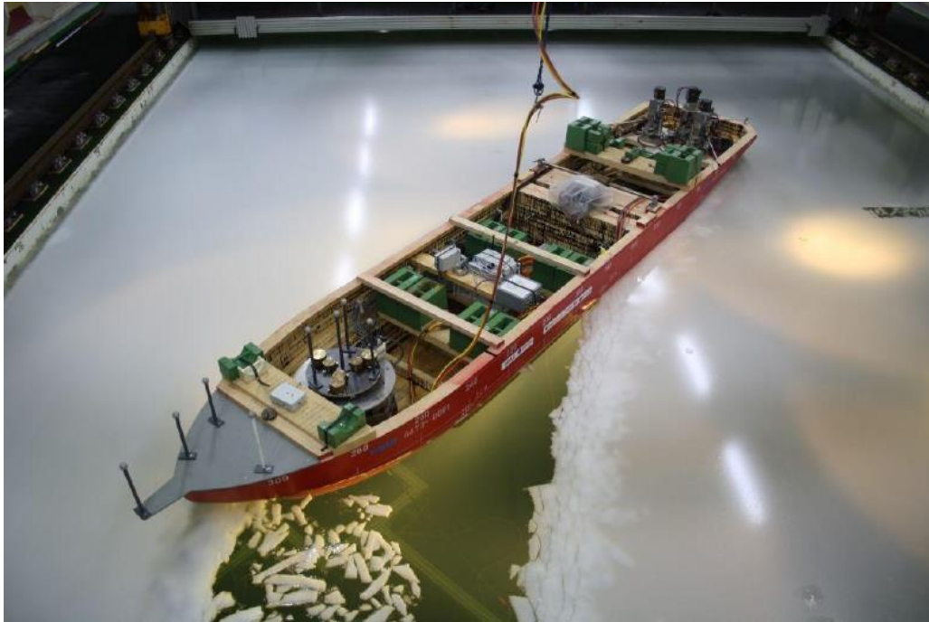
Figure 19. Ice-vaning test with a moored FPU in level ice.
