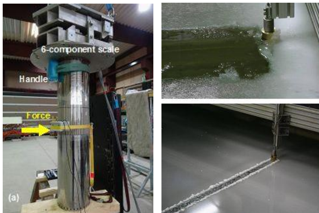
Figure 16. Indenter test with large indenter (diameter 250 mm) outfitted with tactile sensors to measure local ice pressure distribution along the perimeter (a) and small indenter (diameter 60 mm (right).
