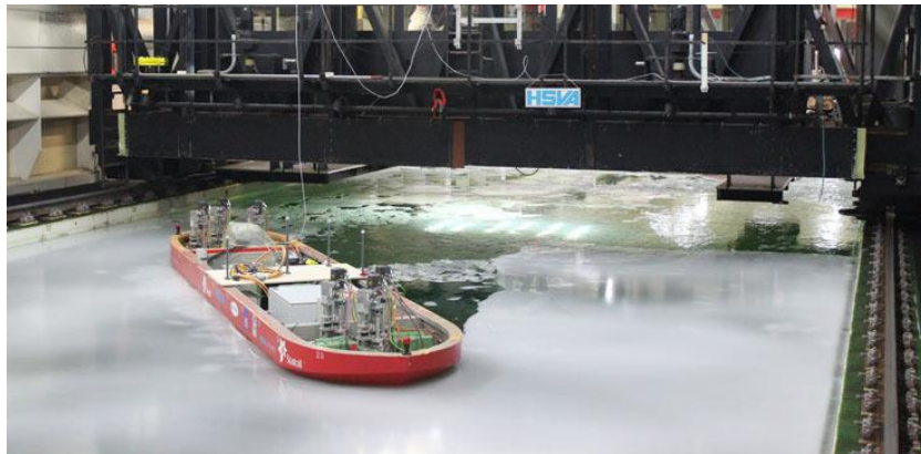
Figure 5. Manoeuvring test of a free running model, model motions in 6-DOF are detected by motion capture system
