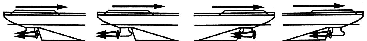
Ahead in pulling mode Ahead in pushing mode Astern in pulling mode Astern in pushing mode Figure 2 Azipod positions and propeller flow directions in different propulsion modes.
